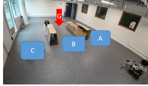
Fig. 8. Real environment setup. The blue regions marked as A, B, C are possible positions of MOs. The red arrow with G is the goal.
